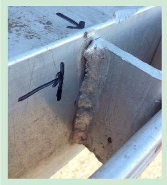
Here is a picture of a flatbed trailer. The arrows are pointing to the weld for a stake pocket between the trailer side and rub rail. Can you see any issues with the weld? The weld is not making complete contact with the side of the trailer on the upper part of the weld. Do you take the time to inspect the condition of all anchor points for your tiedowns?
